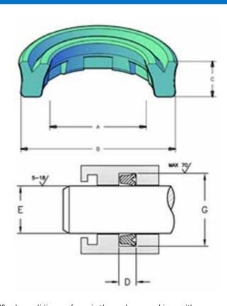
Another contributing factor is the microstructure of the Zurcon U-cup RU9, where sliding surfaces in the seal are combines with back-pumping channels. On the forward stroke of the shaft an oil lubrication film is distributed under the seal. On the return stroke the oil is back-pumped into the system, preventing leakage. This extends seal life by reducing dynamic friction and breakaway force, even after prolonged periods of rest.
