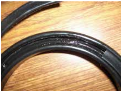
Melted / burned seal material under expander.
