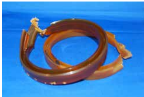
Two piston u-seals exhibiting evidence of pressure trap, air entrapment in seal material and dieseling. Note the burned seal area on the lighter of the two u-seals.
