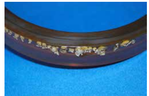
Two piston u-seals exhibiting evidence of pressure trap, air entrapment in seal material and dieseling. Note the burned seal area on the lighter of the two u-seals.
